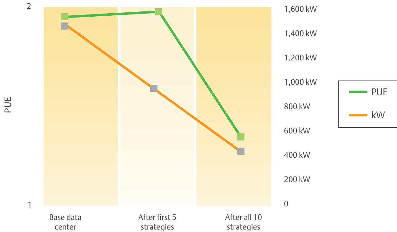
Figure 14. The first five strategies in Energy Logic 2.0 produce a dramatic reduction in energy consumption but a small increase in PUE.
