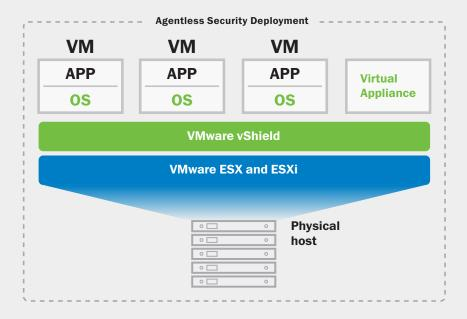
vShield Endpoint uses vSphere 4.1 or 5.0 'plumbing' to deliver the files for inspection to the chosen security appliance.
